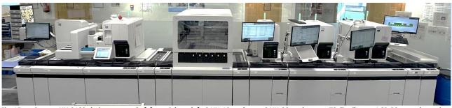
Fig. 15: Sysmex XN-9100 chain composed of, from right to left, 3 XN-10 analyzers; 2 XN-20 analyzers; a TS distributor; 1 SP-50 extender-stainer and a Cellavision ® DI-60
